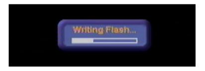
Once the update is complete, the receiver is re-initialised and starts operation again. Never turn off the receiver during the update process, as otherwise you could lose the entire software. If this happened, the receiver would have to be re-installed at a workshop or using a PC and USB cable. On the "STB Management" - "System Information" menu you can see whether the new software has been installed.
